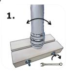
Use an open-end or ring spanner to install the support clamp below the connection. Lower the support clamp in centered position onto the sleeve pipe. Wiggle the riser pipe section and then use the wooden-handled removal tool (included in scope of supply) or a wood screw to pull out the wire spiral.
