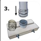
Clean all foreign material off of the jointing surfaces of the connection. Grease the outside surface of the spigot and the inside surface of the socket. Place the "O" ring in the upper groove of the spigot. Then grease the "O" ring. Lower the pipe, again making sure to mate the key and the slot of the anti-twist lock. Complete the connection by completely inserting the retaining wire spiral.
