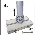
After having inserted the wire spiral, lift the pipeline slightly and remove the support clamp.
