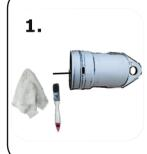
Using a clean cloth or brush, grease the inside of the hoisting socket. The hole at the end of the hoisting socket permits fastening to the shackle on your crane's lifting cable.
