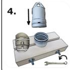
Now put the hoisting socket onto the next riser pipe section, again making sure to mate the key and the slot of the anti-twist lock. Complete the connection by inserting the wire spiral. Lift the riser pipeline slightly and remove the support clamp. Now lift the riser pipeline one pipe-section length upwards and repeat these steps 1 through 4.
