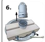
Using an open-end spanner or spanner, install the support clamp below the connection. Lower the support clamp in a centered position onto the sleeve pipe. Wiggle the hoisting socket briefly and then pull out the wire spiral. pull off the hoisting Then socket and slide it in place on the next pipe section.
